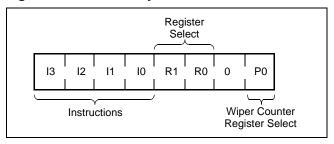
The four high order bits define the instruction. The next two bits (R1 and R0) select one of the four registers that is to be acted upon when a register oriented instruction is issued. The last bits (P0) select which one of the two potentiometers is to be affected by the instruction. Bit 1 is defined to be 0.
