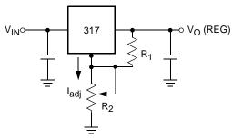
$V_O (REG) = 1.25V (1+R_2/R_1)+I_{adj} R_2$
