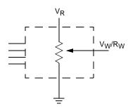
Three terminal Potentiometer; Variable voltage divider
