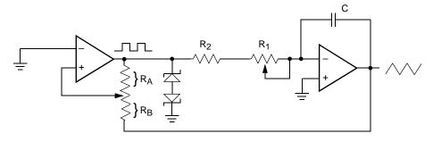
$\begin{array}{l} \text{frequency} \propto R_1,\,R_2,\,C \\ \text{amplitude} \propto R_A,\,R_B \end{array}$
