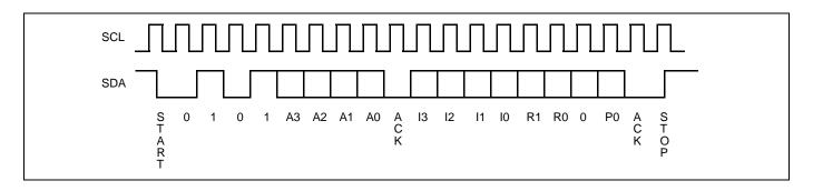
The Increment/Decrement command is different from the other commands. Once the command is issued and the X9418 has responded with an acknowledge, the master can clock the selected wiper up and/or down in one segment steps; thereby, providing a fine tuning capability to the host. For each SCL clock pulse ( $t_{\mbox{HIGH}}$ ) while SDA is HIGH, the selected wiper will
