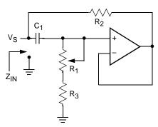
$Z_{1N} = R_2 + s R_2 (R_1 + R_3) C_1 = R_2 + s Leq (R_1 + R_3) >> R_2$
